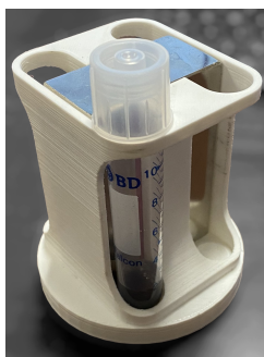
Fig. 7. Simple MP separator made using a permanent magnet block and a 3D printed housing.
